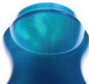
Roll-on deodorant housing molded without Promix Static Mixer 不帶 Promix 靜態混合器的滾珠式除臭劑外殼成型
