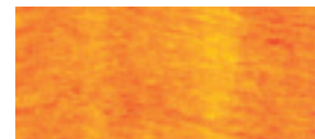
Thermoscan of a PE-coating film with Promix Melt Blender 使用 Promix 熔體混合器對 PE 塗層薄膜進行熱掃描
